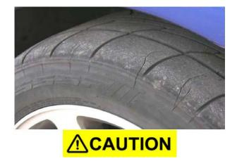
The rubber compounds used in these tires have unique properties that, when compared to other tires, can cause them to lose some of their flexibility when used or handled in conditions below 15°F (-9°C). This loss in flexibility can lead to potential cracking and other damage to the tire.
