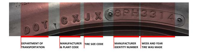
Prior to 2000, the year code of the manufacture date was represented by 1 digit instead of 2 (*i.e.*, 378 would represent the 37<sup>th</sup> week of 1998). In the absence of the decade triangle, this tire would have been made during the 37<sup>th</sup> week of 1988.
