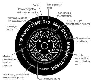
The letters "DOT" certify compliance with all applicable safety standards established by the U.S. Department of Transportation (DOT). Adjacent to this is a tire identification or serial number. This serial number is a code with up to 12 digits that are a combination of numbers and letters. The last characters are numbers identifying the week and year of manufacture. (For example, "1502" means the fifteenth week of the year 2002.)
