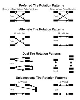
Full-size spare tires (not temporary spares) of the same size, construction, and speed rating may be used in a five-tire rotation pattern.
